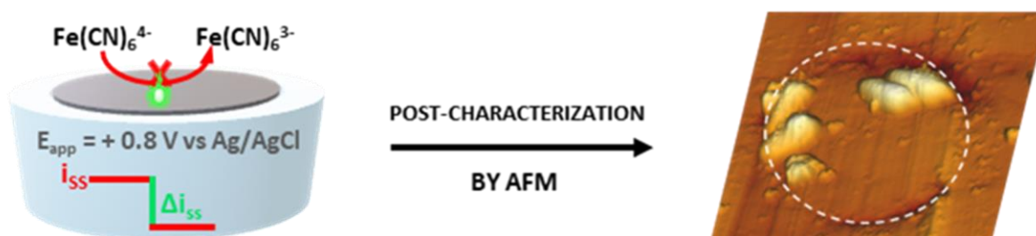
Figure. Single electrochemical impacts of Shewanella oneidensis onto an ultramicroelectrode polarized at the oxidation potential of the ferrocyanide redox probe in solution and post-characterization of the bacteria adsorption onto the electrode surface by atomic force microscopy [2].
