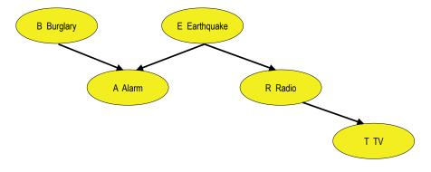
$$P(B, E, A, R, T) = P(B) \times P(E|B) \times P(A|B, E) \times P(R|B, E, A) \times P(T|B, E, A, R)$$
