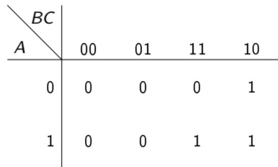
$$f(A, B, C) = \overline{AB}\overline{C} + A\overline{B}\overline{C} + ABC$$
