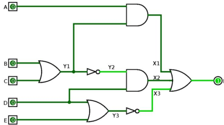
$$\begin{aligned}F &= X_1 + X_2 + X_3 \\&= A \times Y_1 + Y_2 \times D + \overline{Y_3} \\&= A \times (B + C) + \overline{Y_1} \times D + \overline{D + E} \\&= A \times (B + C) + \overline{B + C} \times D + \overline{D + E}\end{aligned}$$
